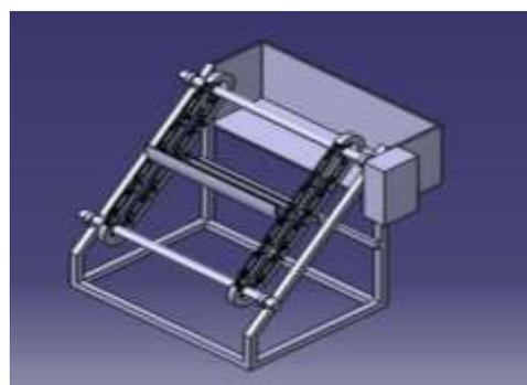
Fig.10: 3-D Model of automatic drain cleaner
