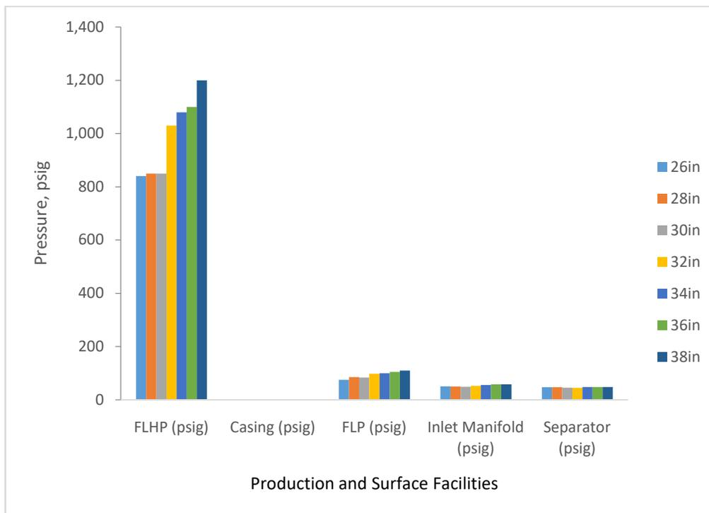
**Figure 3.1: Pressure Measurements of Production and Surface Facilities for the Seven Different Choke Sizes**
