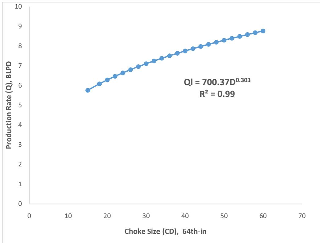
**Figure 3.3: Q (Flow Rate) against CD (Choke Size)**
