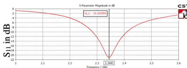
Figure 12: The simulated return loss of the antenna implanted on pleura and lungs for the case stage 0 tumors
