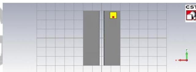
Figure 4: Patch antenna implanted on pleura and lungs
