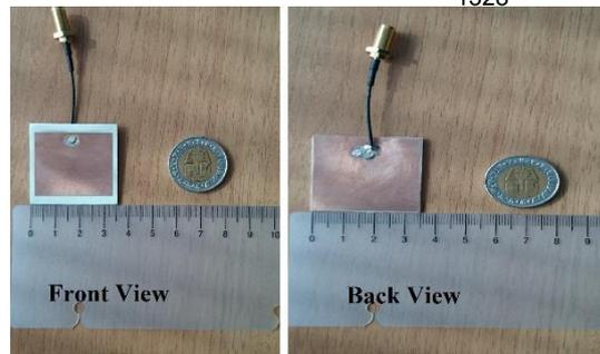
Figure 2: Fabricated antenna
