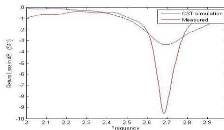
Figure 10: Simulated and measured return loss of patch antenna in free space.
