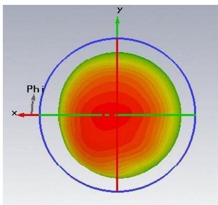
Figure 7: 3D radiation pattern of patch antenna.
