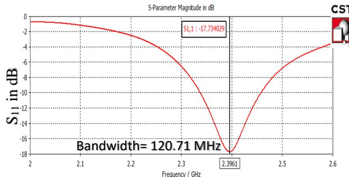
Figure 24: The simulated return loss of the antenna implanted on pleura and lungs for the case stage IV tumors
