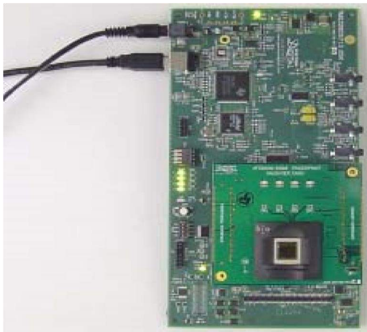
Figure 3: FDC-AFS8600 Sensor Board Mounted on C6713 DSK
