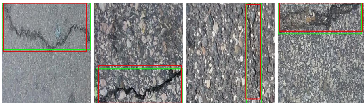
Fig. 7. Ground-truth (green) and predicted (red) bounding boxes under diverse surface textures and illumination conditions.
