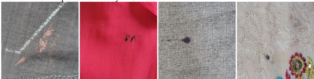
Fig. 4. Representative samples of spot defects from the FabricSpotDefect dataset.
