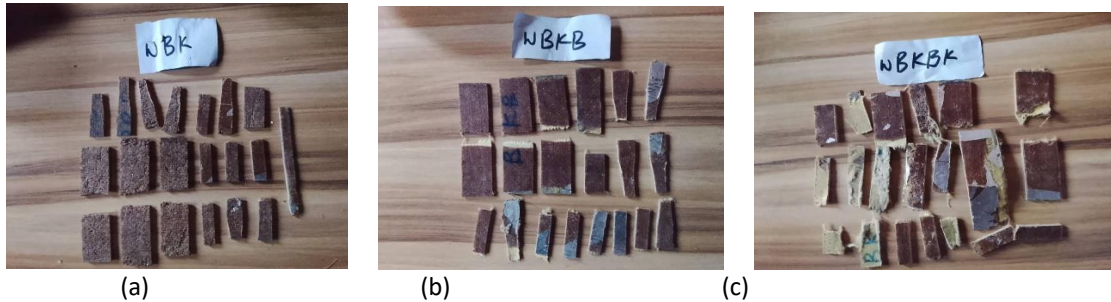
Figure 6: (a) One layer of woven-Bamboo and Kevlar. (b) Two layers of Bamboo with Kevlar in-between. (c) Two layers of Bamboo and Kevlar in-between each other
