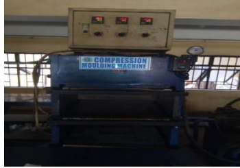
Figure 2: Compression Moulding Machine for curing of the composite samples
