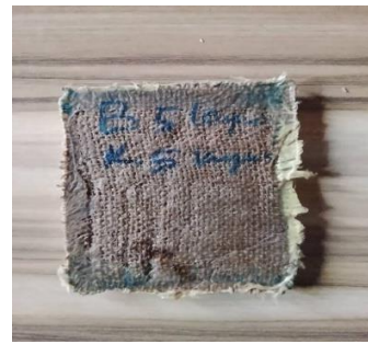
Figure 8: Compressed ten (10) layers of woven-bamboo fibers and Kevlar
