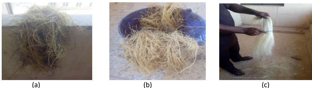
Figure 1: (a) Raw Extracted Fiber from Bamboo. (b) Bamboo Fiber in Process of treatment. (c) Combing/brushing of the treated Bamboo Fiber.
