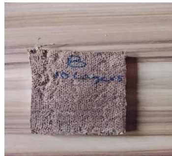
Figure 7: Compressed ten (10) layers of woven-bamboo fibers only.
