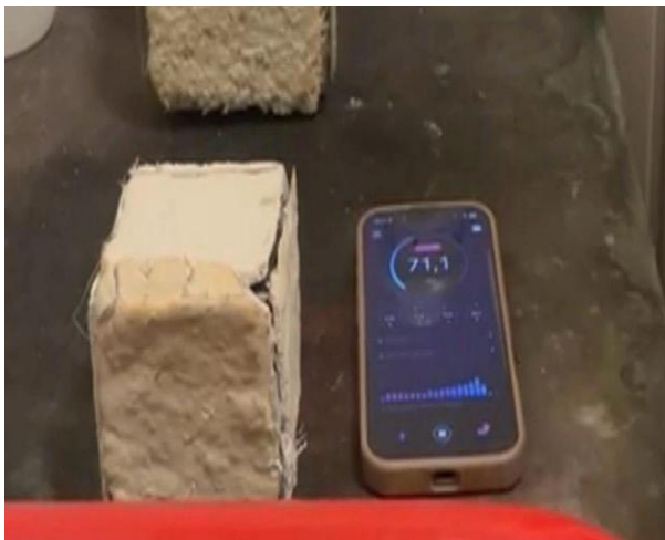
Figure 2.4.1. Measurement from the NaOH-based panel
