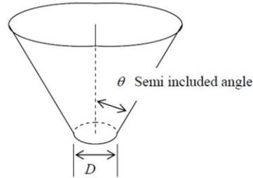
Figure 13: Conical hopper with outlet size,  $D$ , and semi included angle  $\theta$ .
