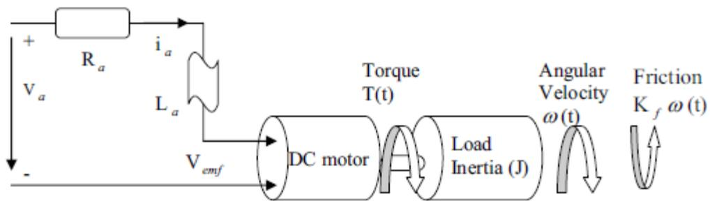
Figure 15: General model of DC motor [37]
