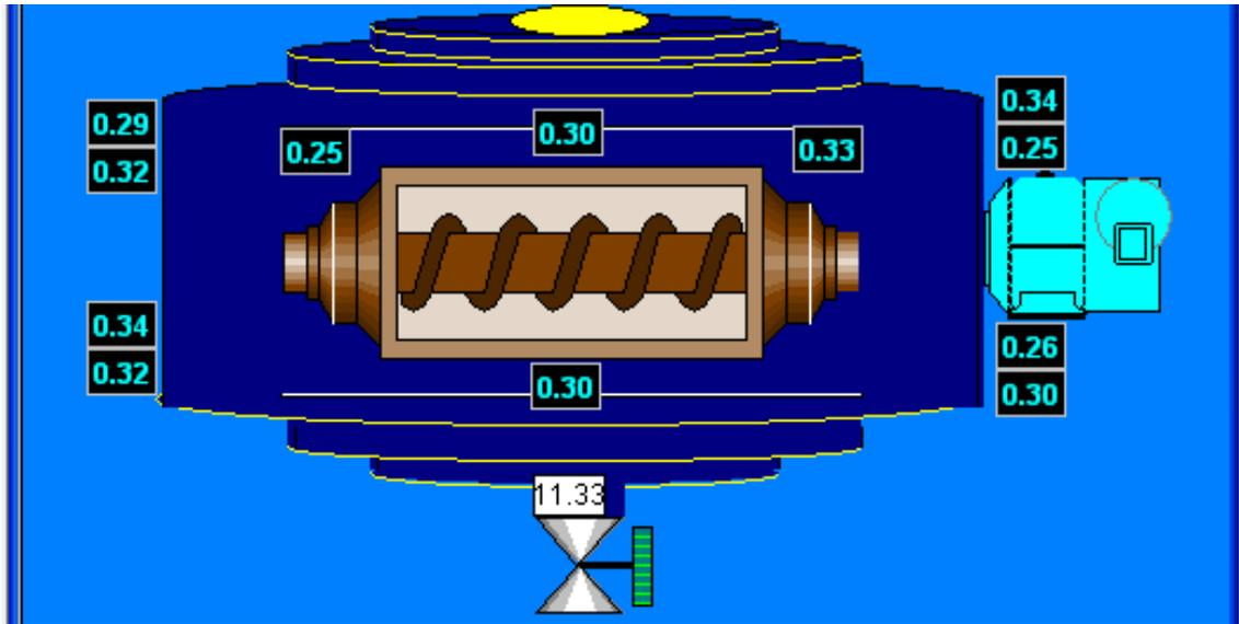
Plate XV: HMI display for the location of the Virtual sensor probes on the sides of the mixing chamber
