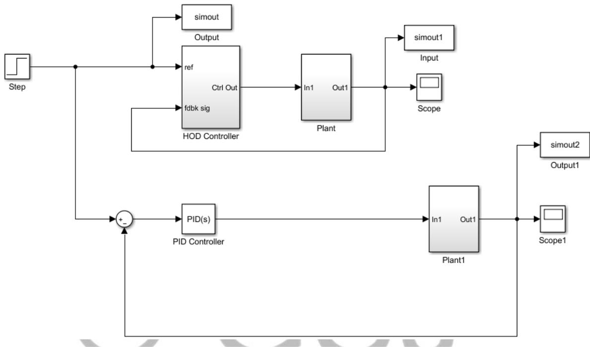
Figure 17: Simulink representation for the two the controlled closed loop of the system, one with PID controller and another with HODFC.
