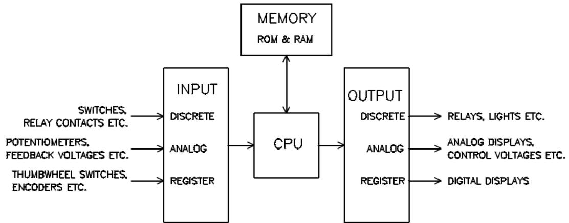
*Figure 8: Programmable Controller Block Diagram*
