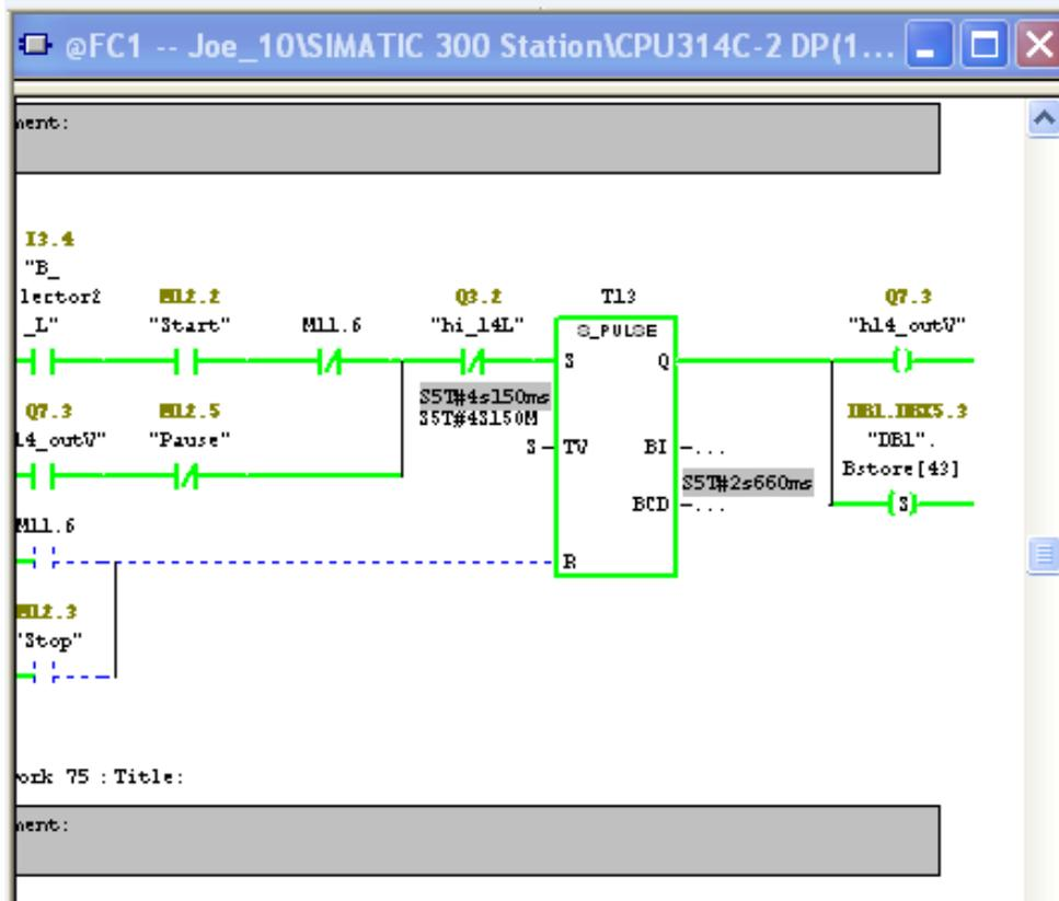
Plate II: Program that executed opening of hopper 14 discharge valve and times out its closing for estimated mass to be discharged.
