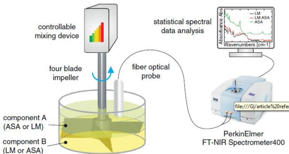
Figure 7: Schematic of the experimental setup with a four-bladed mixer connected to a controllable mixing device. The fiber optical reflectance probe of the FT-NIR spectrometer was in direct contact with the powder during the mixing process[44] .
