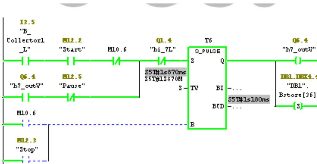
Plate III: Execution of Hopper 7 discharge timing
