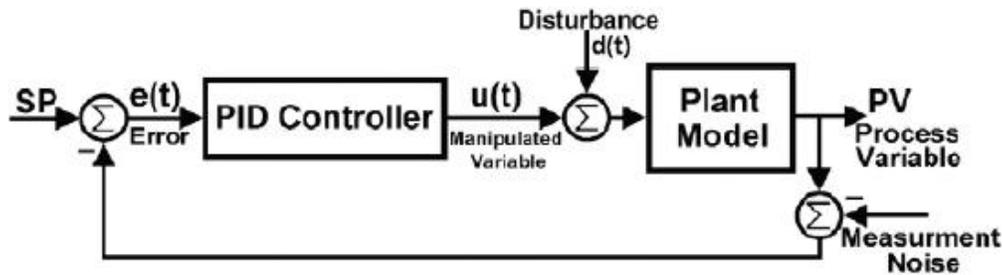
Figure 16: A typical PID control structure
