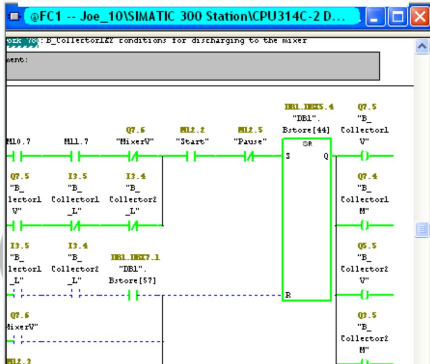
Plate V: Program executing discharge from the two big collector hoppers into the mixing chamber.
