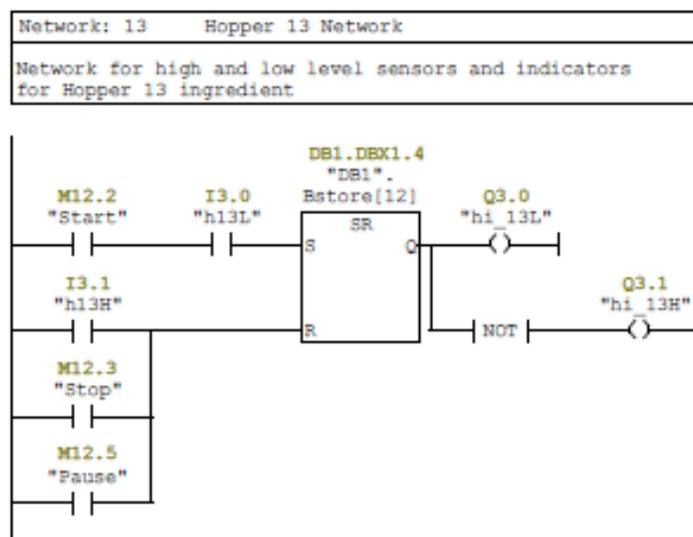
Figure 11: Program for High and Low level sensor indicator
