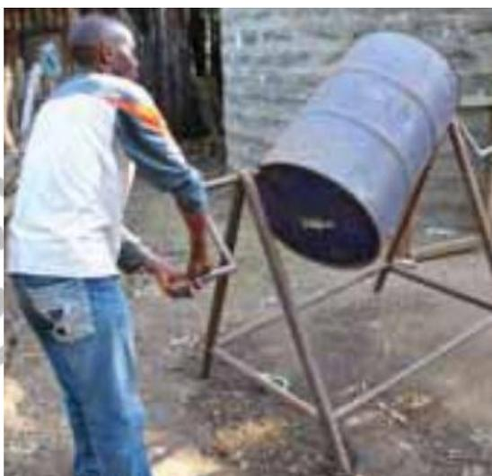
*Figure 3: Mixing feed with drum mixer .*
