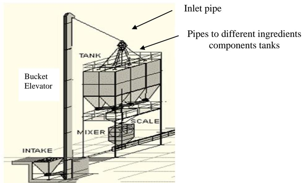
*Figure 1: Feed Production Process*
