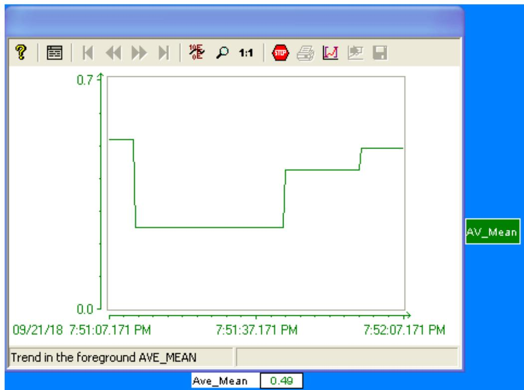
Plate XVI: HMI real-time update plotting of the average cumulative Mean for the four Channels until set point ( $F_{CV} \leq 4.00$ ) is reached.
