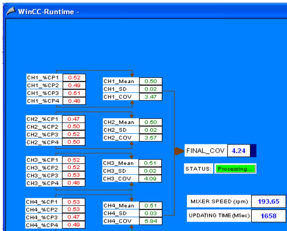
Plate XII: HMI simulations for all the process readings
