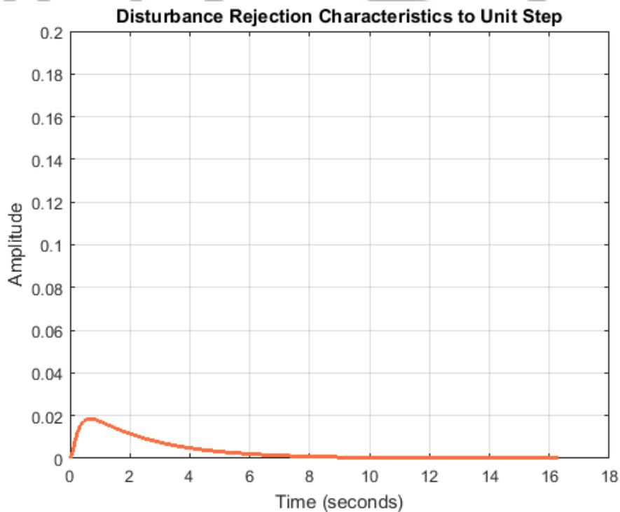
Figure 23: PID controller disturbance rejection for the plant
