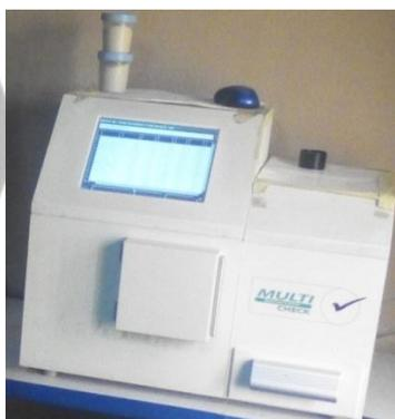
*Figure 4: Multi check NIR spectrometer [14].*
