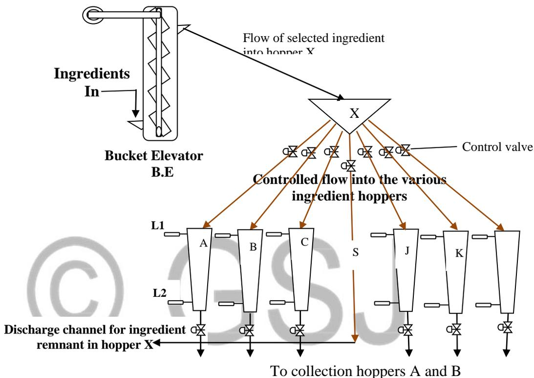
Figure 10: Schematic Flow Pattern from B.E to the Individual Hoppers
