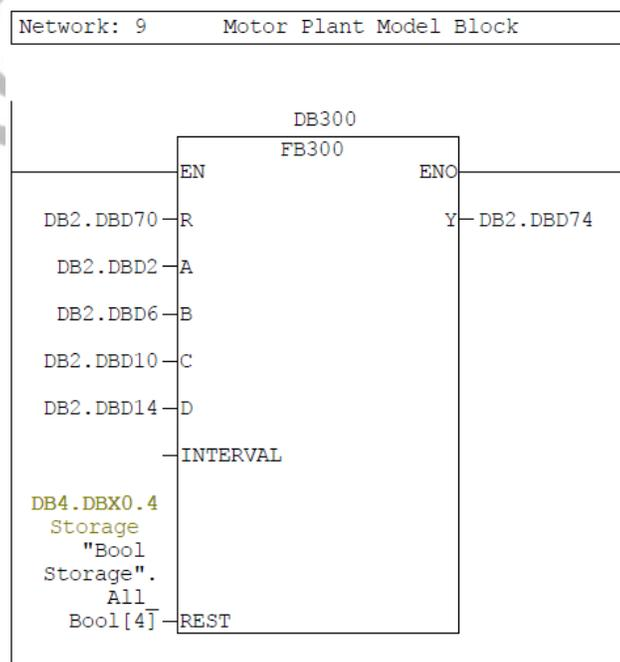
Figure 46: Plant model block
