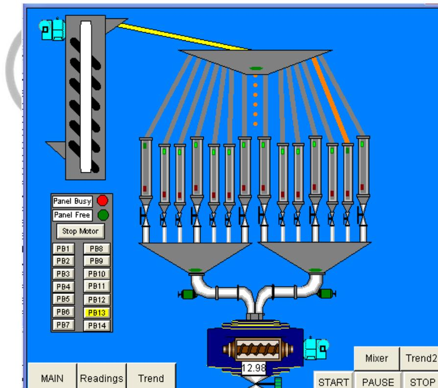
Plate I: HMI Process implementation of the program designed
