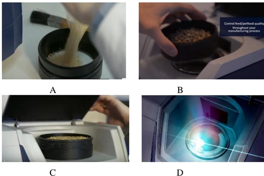
*Figure 6: Sample mixed feed in sample thief and Near Infrared Spectrometer[15]*
