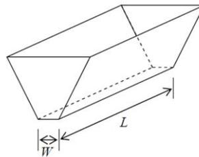
Figure 14: Symmetrical slot outlet hopper of opening size  $W \times L$ .
