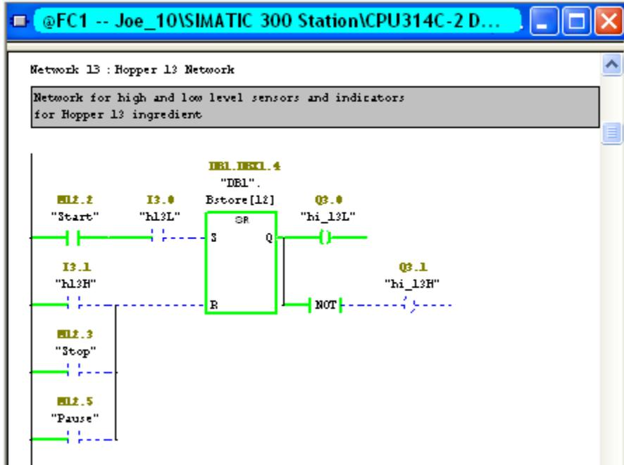
Figure 20: Simulation for low level sensor indicator for hopper 13 activated
