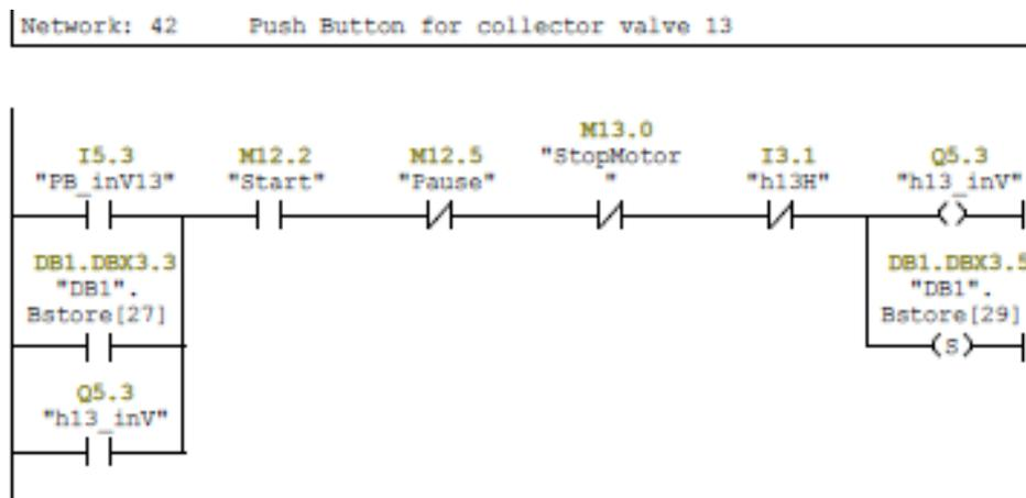
Figure 12: Program to active the opening of hopper 13 valve by press the push button
