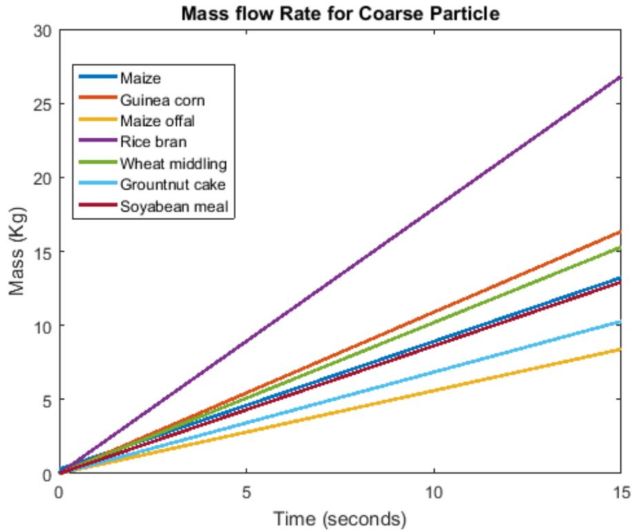
Figure 24: Mass flow rate for Coarse particles
