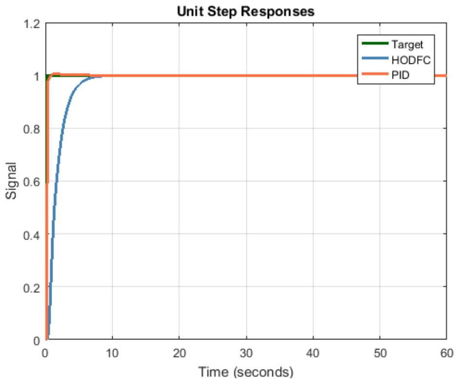
Figure 22: The Responses of the two controllers on the system
