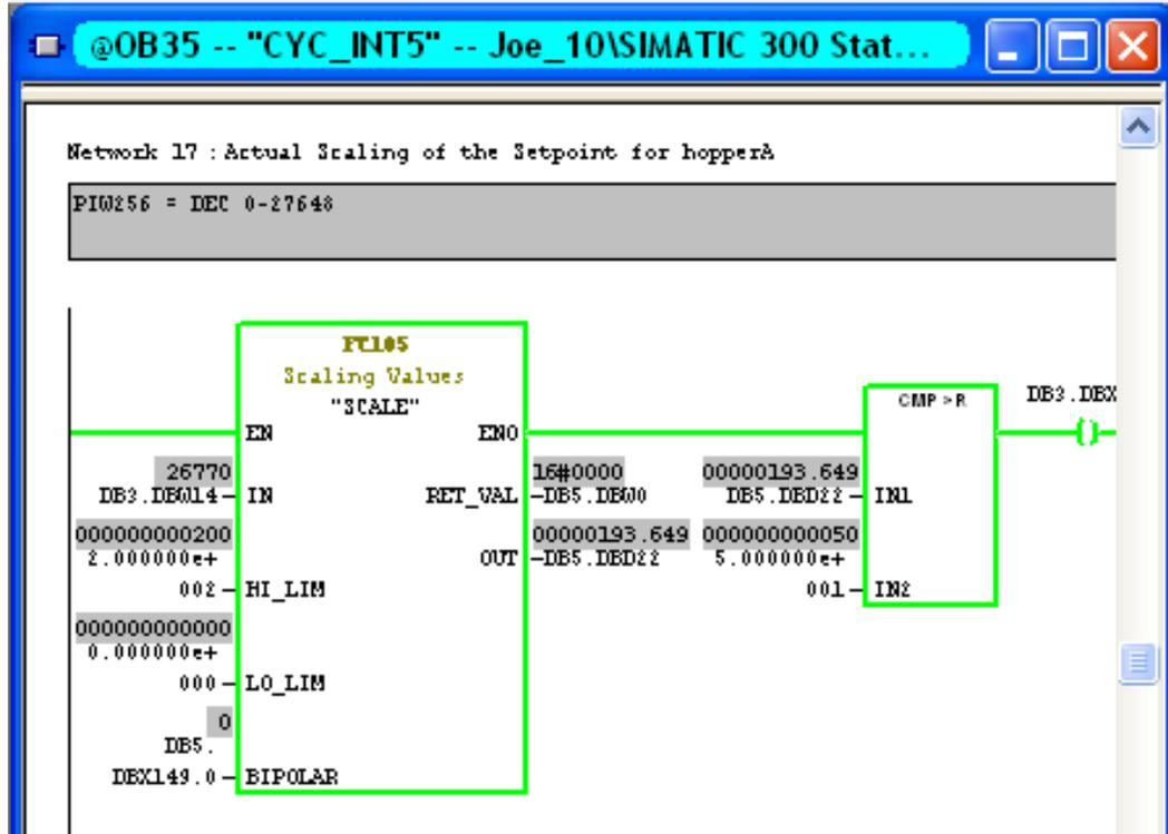
Plate VII: Actual scaling of the speed limit
