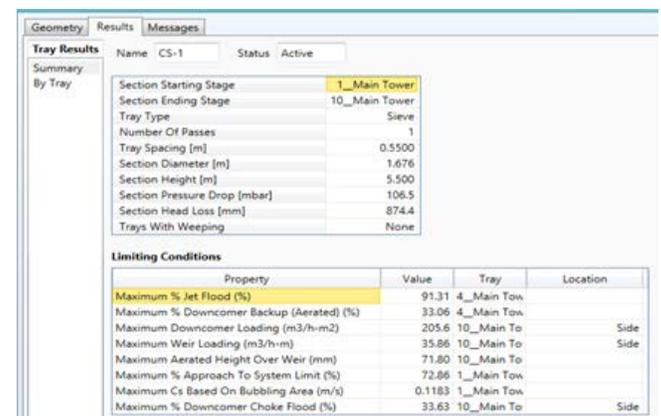
Fig 6 and 7 Show the distillation column sizing result obtained using Aspen HYSYS. The column geometry, internals results are shown
