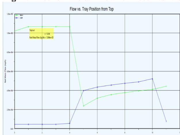
Fig 4 Shows the flow of liquid and vapour at the various stages in the column
