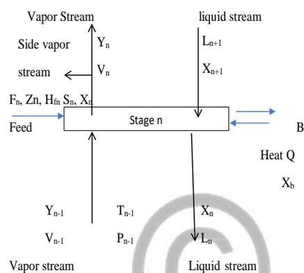
**Fig 2. Multicomponent distillation Column diagram for stage n (Feed)**
