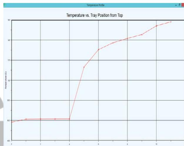
Shows the Temperature vs Tray position from top. The graph shows the uneven distribution of the temperature across the distillation column.
