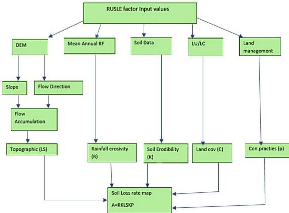
Figure 3:12 Framework to estimate Soil Erosion Rate and Map Using USLE Model in A GIS
