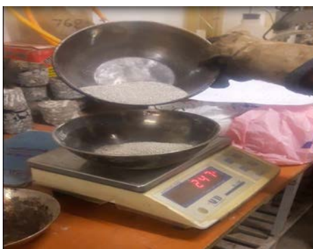
Figure: 2 weighing of required material for single mould
