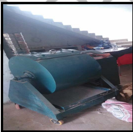
Figure:9 Los-Angeles abrasion drum
