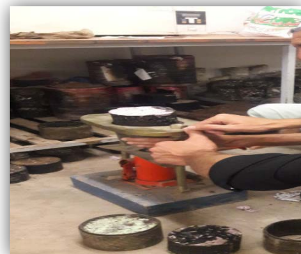
Figure: 3 extractions of mould after preparation and cooled at room temperature
