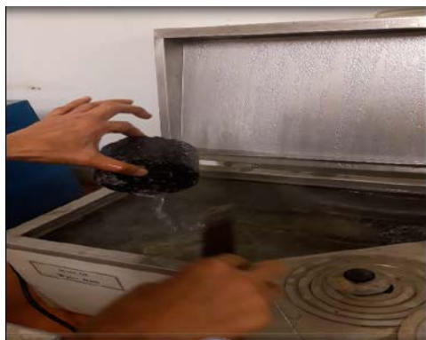
Figure: 4 moulds are kept at 60°C for 1 hr.
