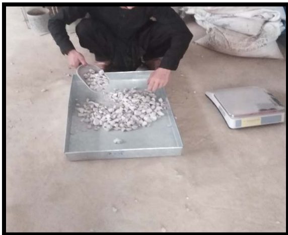
Figure: 10, Sieve analysis of coarse aggregates
