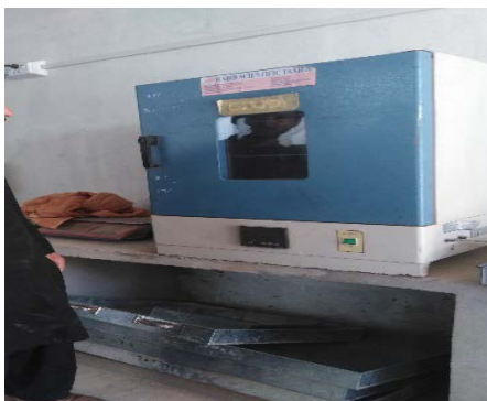
Figure: 1 placing of aggregate for 1hr at 160°C
