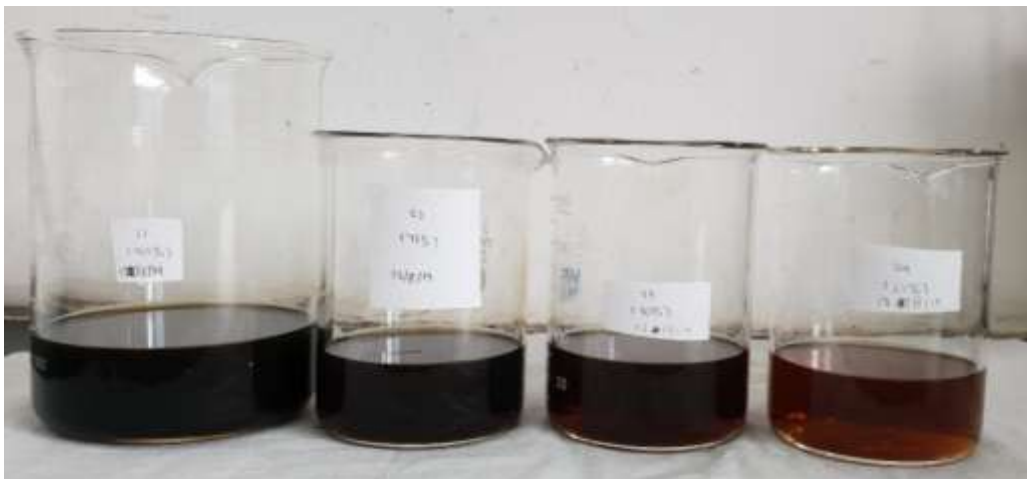
Figure 1. Standard solutions. From left: S1(100%), followed by S2(75%), then S3(50%) and S4(25%)
