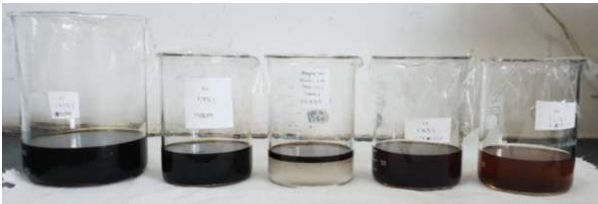
Figure 5. Colour comparison of Mixture M (DOR 1:20) with standard solutions
