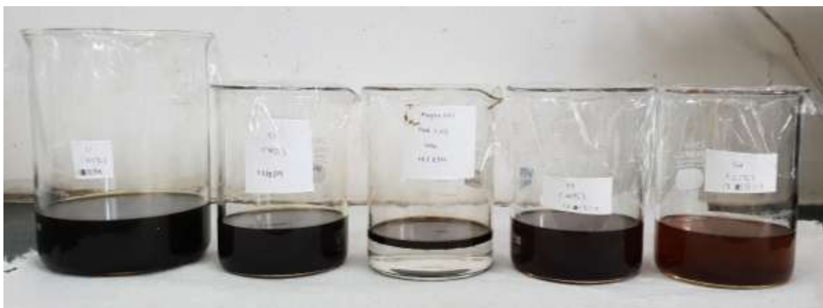
Figure 3. Colour Comparison of Mixture M (DOR 1:20) with standard solutions
