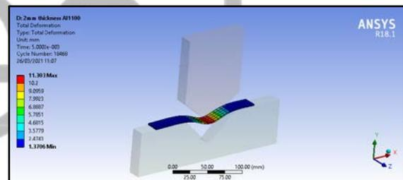
Figure 10: deformation at 0.5 ms
