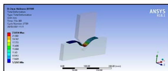
Figure 12: deformation at 0.75 ms
