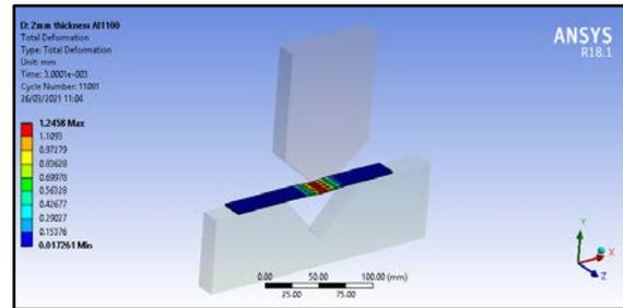
Figure 8: Deformation at 0.3 ms
