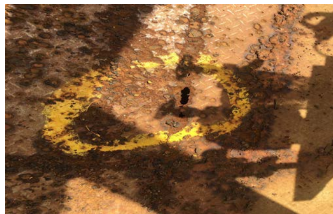
Plate 4: Corroded deck plate surfaces at FPSO front puffin Source: Researchers Field survey, 2021
