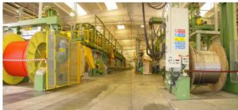
Fig. 9 One shot production: from conductor to finished cable without any interruption
