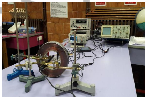
(The magnetic coil, the petri dish containing the HeLa cell culture and the signal generator are visible.)
