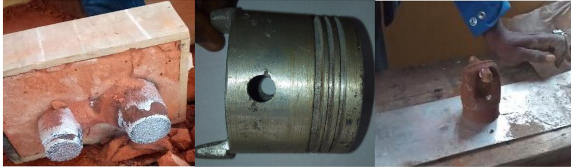
**Plate 2.1** Photographic view of some of the processes followed to produce the piston
