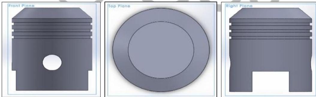
Fig. 2.4: Orthographic view of modelled piston
