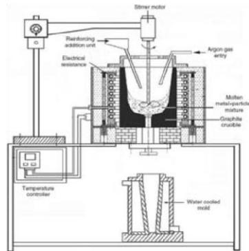
**Fig. 2.1: Electrical Furnace Used for the Preparation of the Specimen**
