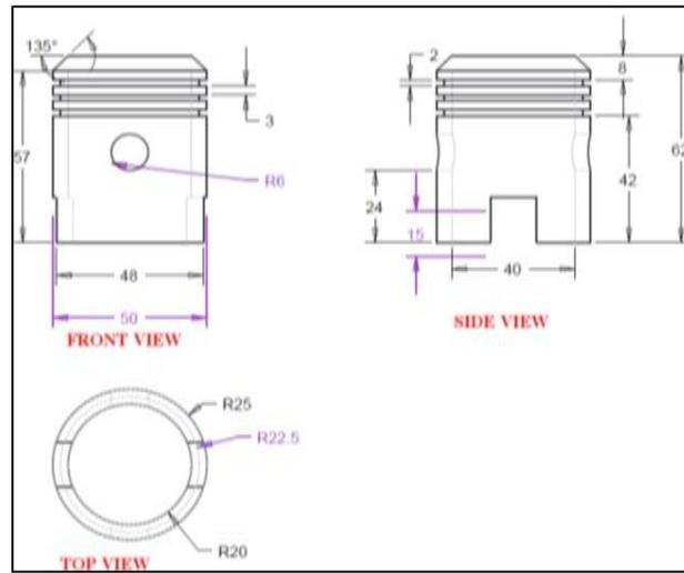
Fig. 2.2: Engineering drawing of a piston
