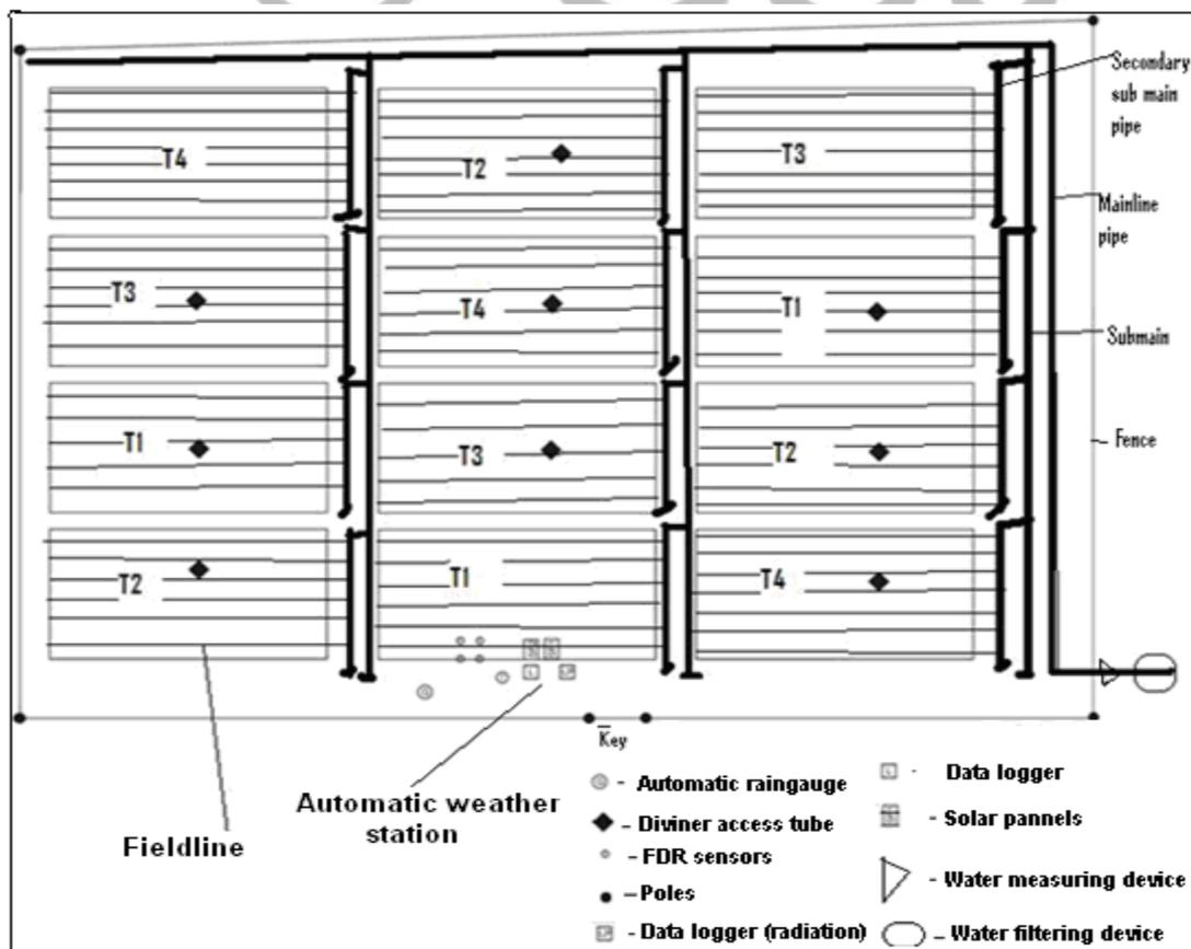
Figure 3: Sketch of the experimental set up at SUA Morogoro
