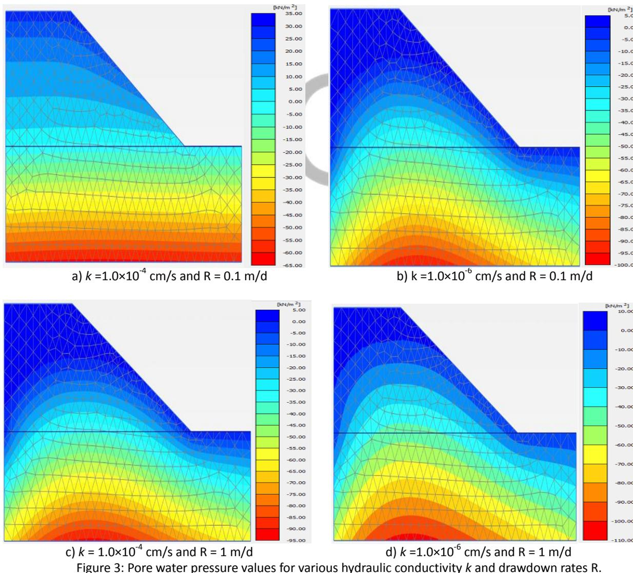
Figure 3: Pore water pressure values for various hydraulic conductivity  $k$  and drawdown rates  $R$ .
