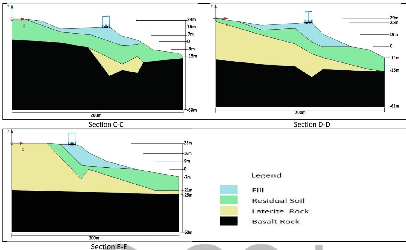
Figure 12: Soil profile at different sections (A-A to E-E).
