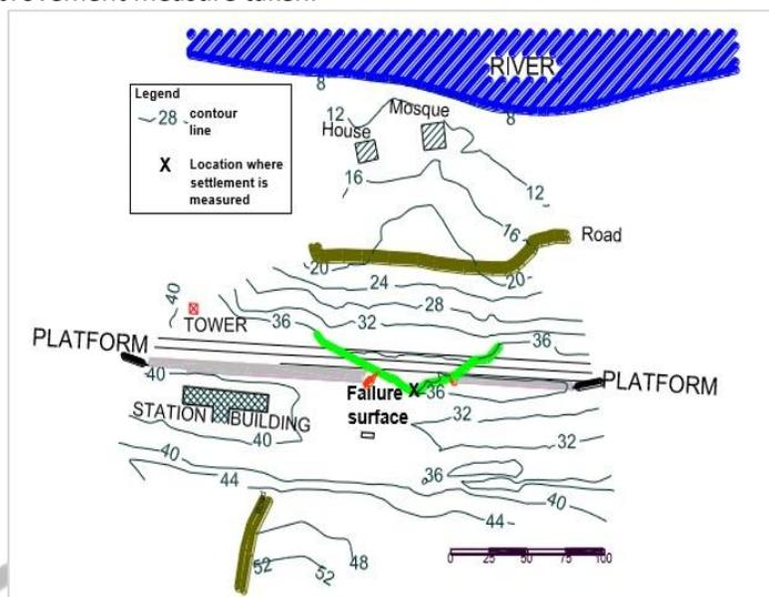
Figure 10: Failure at Nivsar Yard Embankment, [9].
