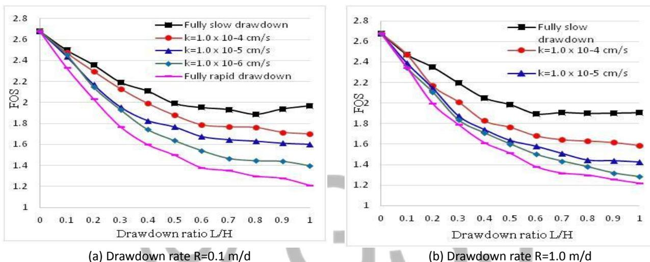
Figure 4: Variation of FOS with drawdown ratio for various hydraulic conductivity  $k$  and drawdown rates  $R$ , (present study).
