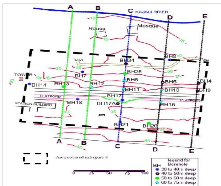
Figure 11: Borehole location along the 5 sections, [9].
