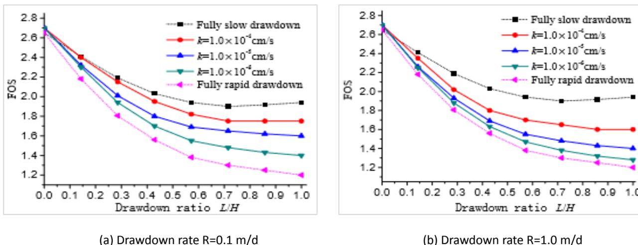
Figure 5: Variation of FOS with drawdown ratio for various hydraulic conductivity  $k$  and drawdown rates  $R$ , [7].
