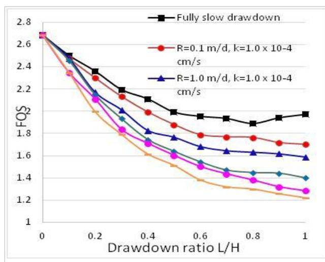
Figure 6: Variation of FOS with drawdown ratio for Various drawdown rates  $R$  and hydraulic conductivity  $k$ , (Present study).
