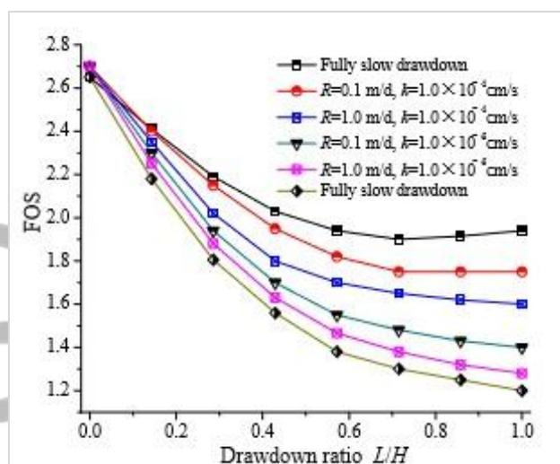
Figure 7: Variation of FOS with drawdown ratio For various drawdown rates  $R$  and hydraulic conductivity  $k$ , [7].
