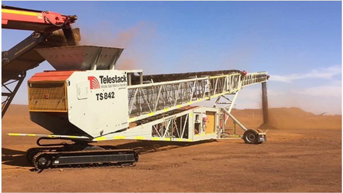
Figure 2: Barge loader/Tele stacker (Source [13])
