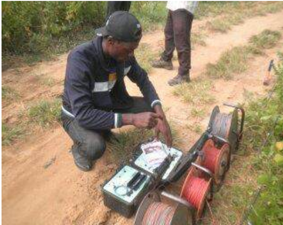
Plate1: showing student conducting electrical resistivity geophysical technique in the study area.
