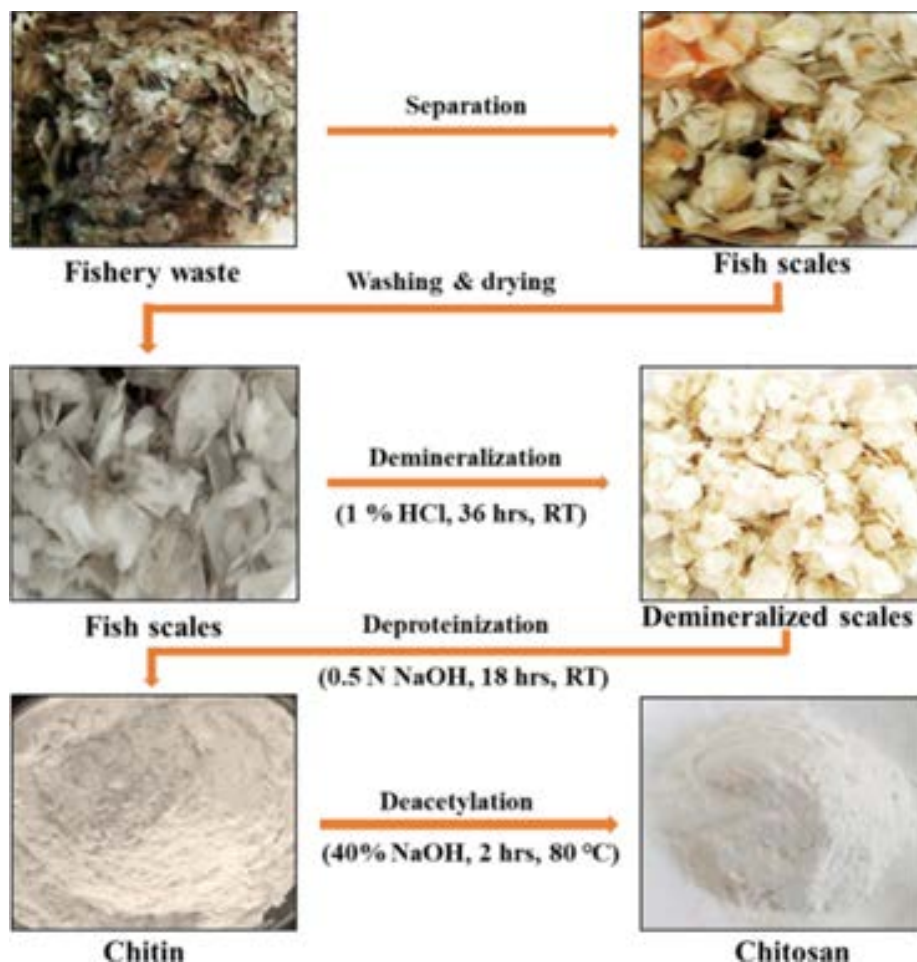
Figure 4. Processes for preparation of chitin from fish scales (Source: Kumar al., 2021)
