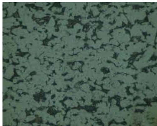
Figure 4. Initial material micro structure of SS 400 steel
