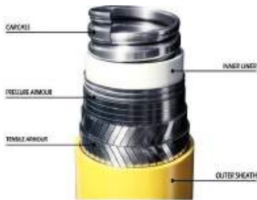
Figure 1: Non-bonded flexible pipe [2]
