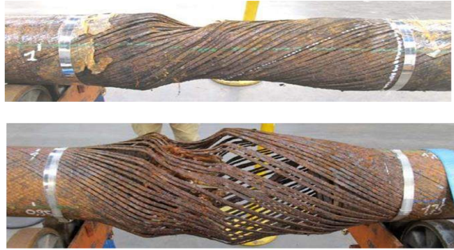
Figure 9: Flowline lateral and radial buckling and blockage
