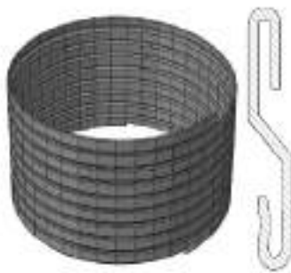
Figure 22: Section and model of carcass layer [21]
