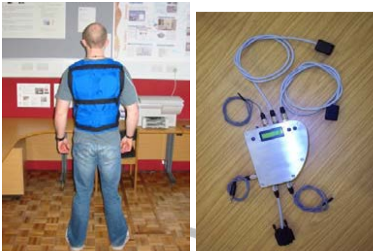
Figure 2: The SensVest - Left the vest and right the electronic enclosure and cable kit. (Woolley, et al, 2003).
